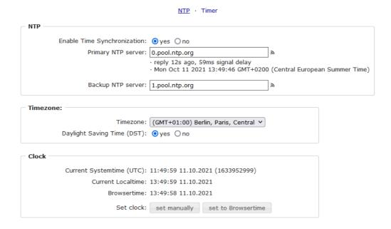
Enable Time Synchronization: Enables the NTP protocol.
