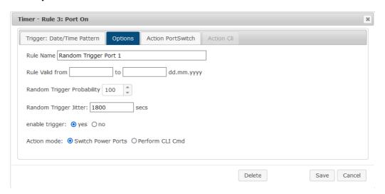
You can use the jitter e.g. for a shutter control. In the classic example of a shutter control, you do not always want to raise and lower the shutters at the same time in order to confuse potential burglars. The jitter of 1800 seconds means that the action is executed randomly in a period between 30 minutes before and 30 minutes after the pro-
