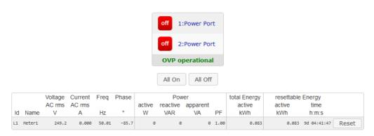
The web page provides an overview of the switching state, energy measurement values, as well as the external sensors, provided that they are connected. The text "OVP operational" indicates that the Overvoltage Protection is working. See chapter Overvoltage Protection 100. When a single port is clicked at the Expert Power Control 1121, a panel with buttons to control a single port appear:
