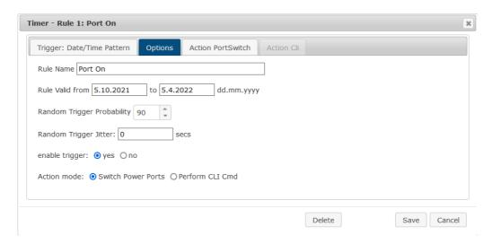
For this rule, on the "Options" tab, the time period is limited to the range between 5.10.2021 and 5.4.2022. In this example, the timer rule is only executed with a probability (Random Trigger Probability) of 90%.
