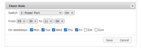
You set here which port should be switched for which time period, and on which days of the week the rule is active. In this example the period 9:00 to 17:00 is changed to 9:30 to 11:00 compared to the default input mask. Also, this rule should not be applied on Saturday and Sunday. The rule we have now says that every day, except Saturday and Sunday, port 1 will be switched on at 9:30 and switched off after 1.5 hours. Clicking on "Save" saves this rule.
