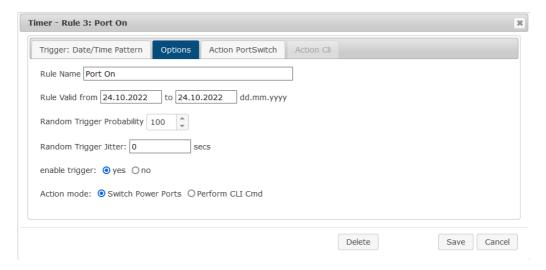
Then call up the two timer rules you created ("On" and "Off") and enter the date on which the switching operation is to take place in the "Options" tab.
