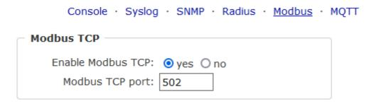
Enable Modbus TCP: Enables Modbus TCP support.
