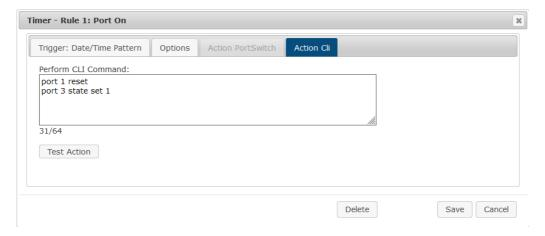
Instead of switching a port, one or more console commands can be executed. These commands are entered in the "Action CLI" register. The "Action Cli" tab can only be selected if the option "Perform CLI Cmd" is activated in "Options".
