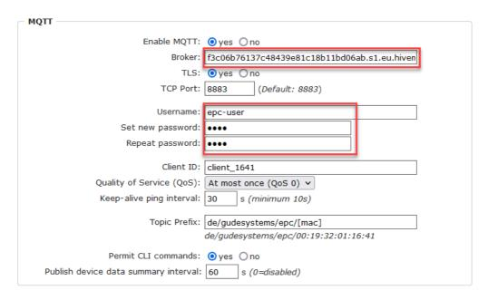
In the MQTT configuration of the Gude device, transfer the hostname of the HiveMQ broker, as well as username and password. Additionally activate TLS and set the correct port.
