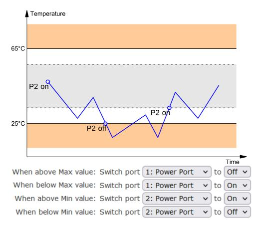
Actions during configuration, device start or plugging in the sensor (for given example):
