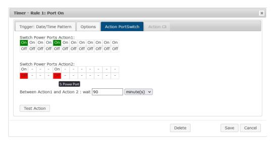
In this example, port 1 and port 5 are enabled and disabled after 90 minutes by batch mode.
