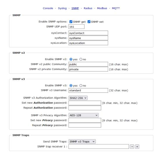
SNMP-get: Enables the acceptance of SNMP-GET commands.
