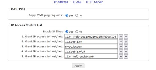
Reply ICMP ping requests: If you enable this feature, the device responds to ICMP pings from the network.
